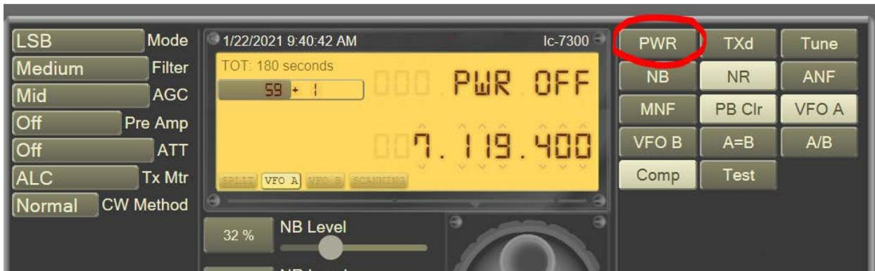
The POWER button has been activated on the WØZSW station interface in version 0.9x of the RCForb software. Please turn the IC-7300 power off when you are finished using the station.
