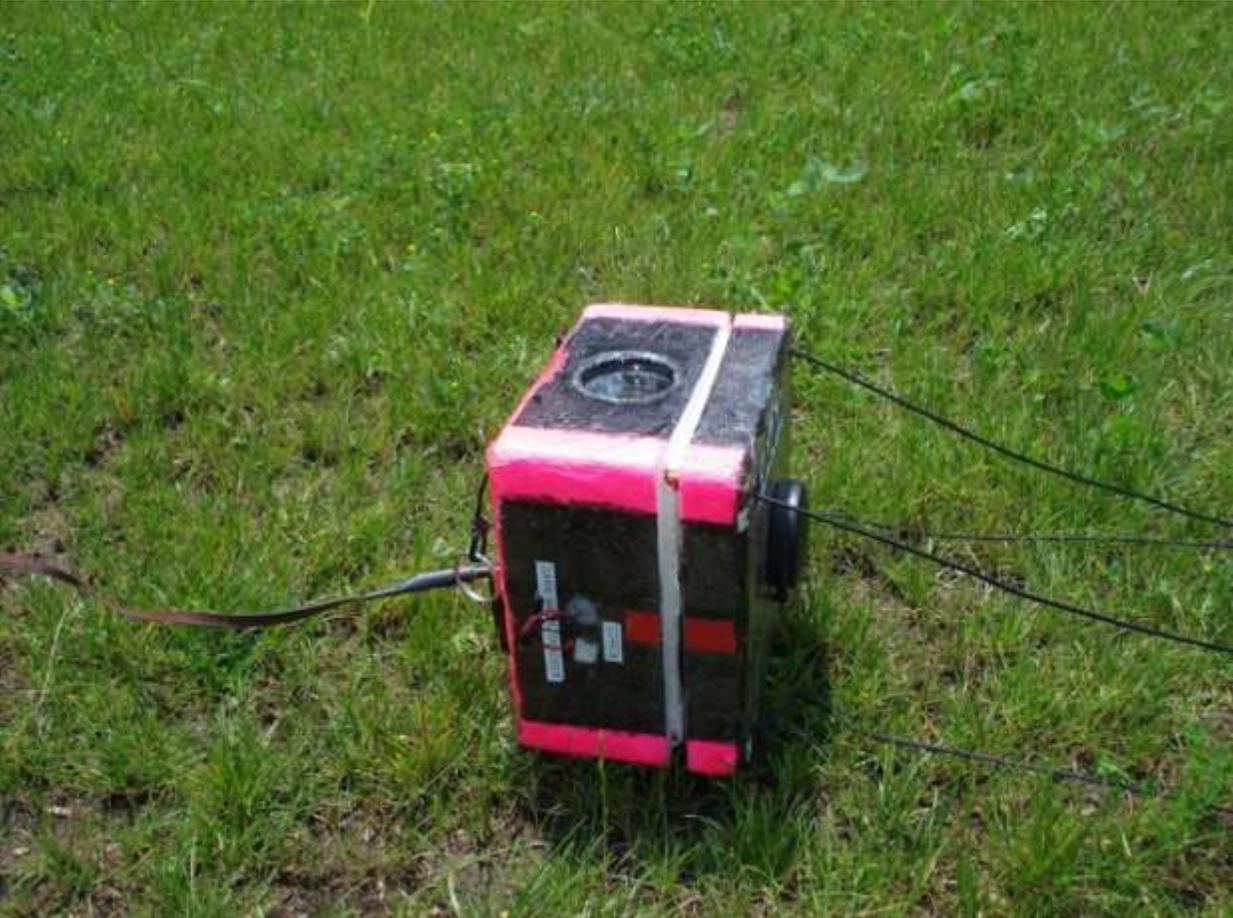
Photo: Payload with APRS prior to flying by WX balloon as SARA partners with U of M students to provide tracking data and assistance.
