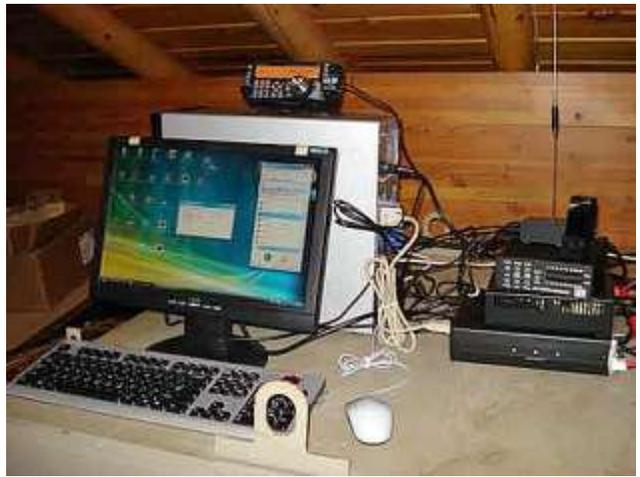
The original WØEQO station, running W4MQ software for rig control and Skype for audio. It was located in an unheated attic in the Courage North camp dining hall, where it ran 24/7/365, providing remote HF access to hams who would not otherwise be able to operate HF.
